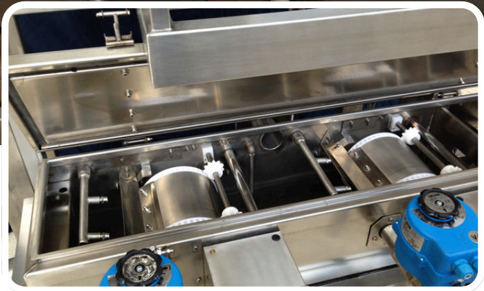
Internal Components of Centralised Auto Skim AGRD
